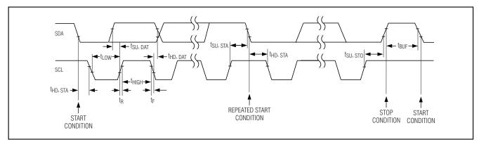
Figure 2. 2-Wire Serial Interface Timing Details
