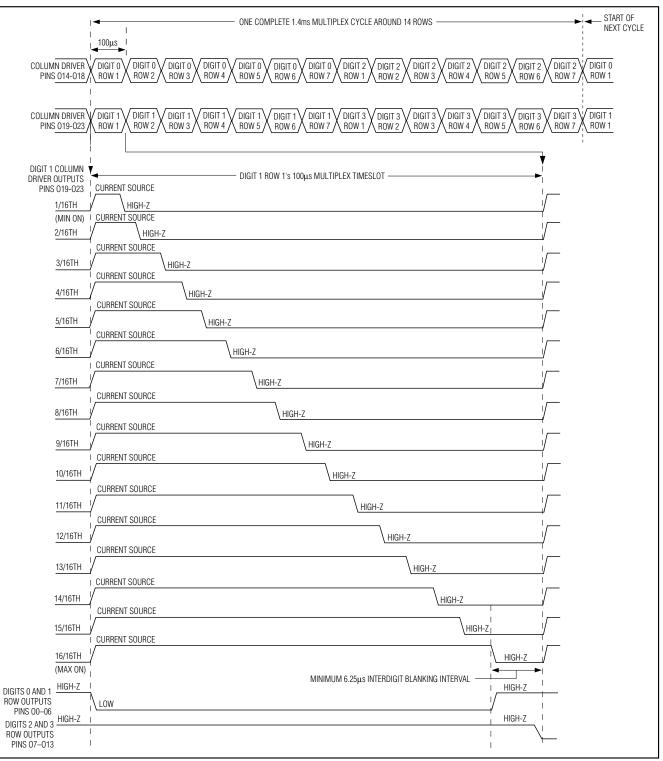
Figure 10. Multiplex Timing Diagram (OSC = 4MHz)
