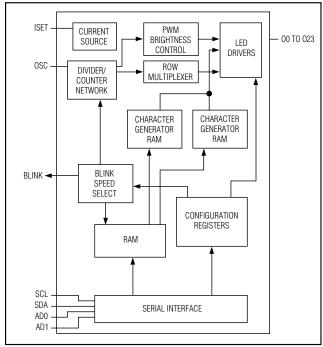
Figure 1. MAX6953 Functional Diagram
