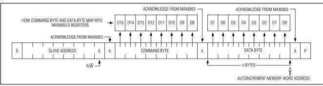
Figure 9. n Data Bytes Received
